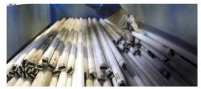
Fluorescent Lamp Recycling This innovative recycling solution separates all geometric shapes of fluorescent lamps into their individual components for recycling and safe disposal.
